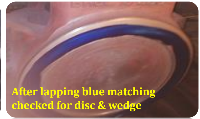
Damaged Seat ring in HWL CV
