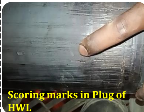
High energy passing valves rectification
